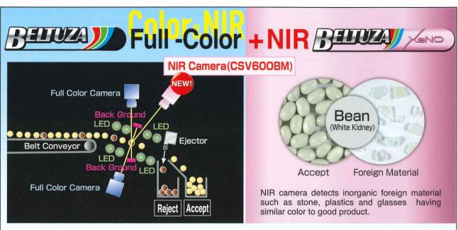
The belt stably and uniformly conveys the material, ensuring high sorting accuracy. The improved LED lightning captures the slightest color differences via sensors. Defective products are ejected from the product stream by air. Detachable components are made of stainless steel for higher hygiene standards.
