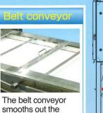
smooths out the material flow, making high capacity delivery possible even for larger materials of irregular shape.
