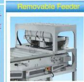
A stainless steel body frame and removable parts provide easy cleaning and sanitation. BELTUZA's vibratory feeder can be removed for flexible product line layout.
