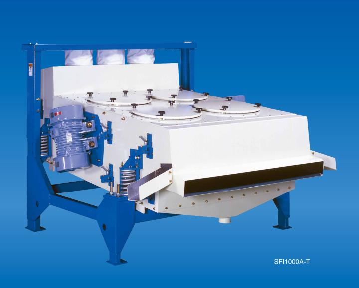
The Satake Milling Separator SFI is an all purpose separator for the cleaning of cereal grains, such as rice, wheat, maize (corn), rye, oats, etc. The oscillation of the double deck sieves efficiently removes both large or coarse material, and fine impurities from the grain being cleaned.
